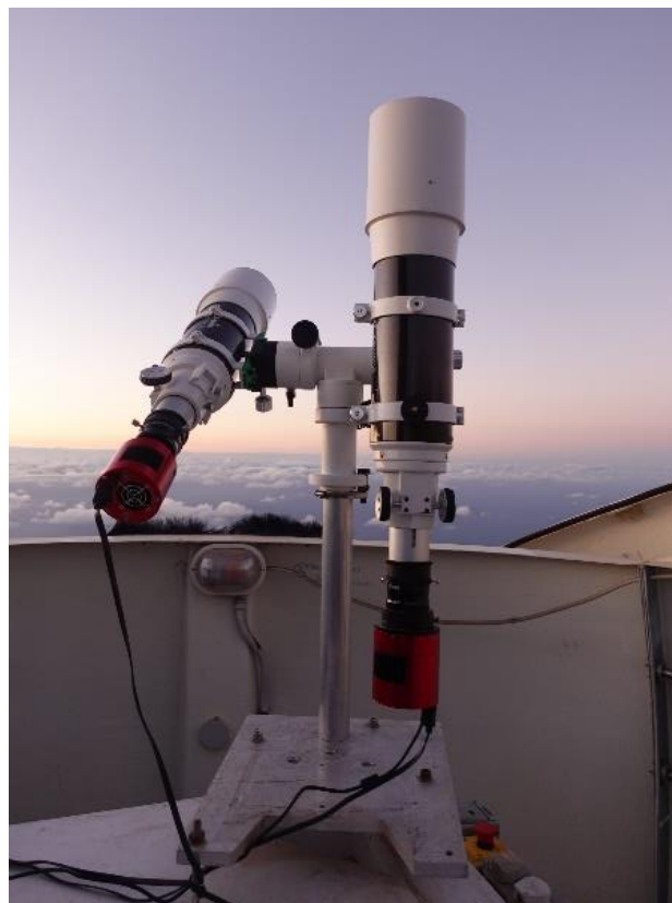
Figure 2: SDIMMs Dual Telescope Setup. Left: Polaris DIMM, Right Zenith DIMM.
